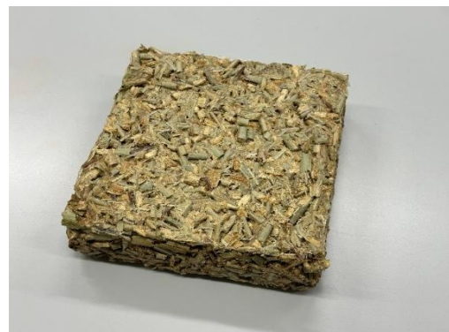
Fig. 7. Sample of the developed thermal insulation material – crushed reeds with carrageenan adhesive; the pores are filled with fine reed particles
