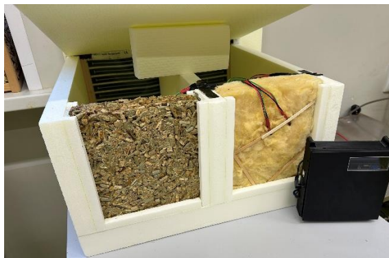
Fig. 6. Experimental setup for heat transfer tests; the test and reference (glass wool) materials are heated equally, and temperature data is obtained on both sides
